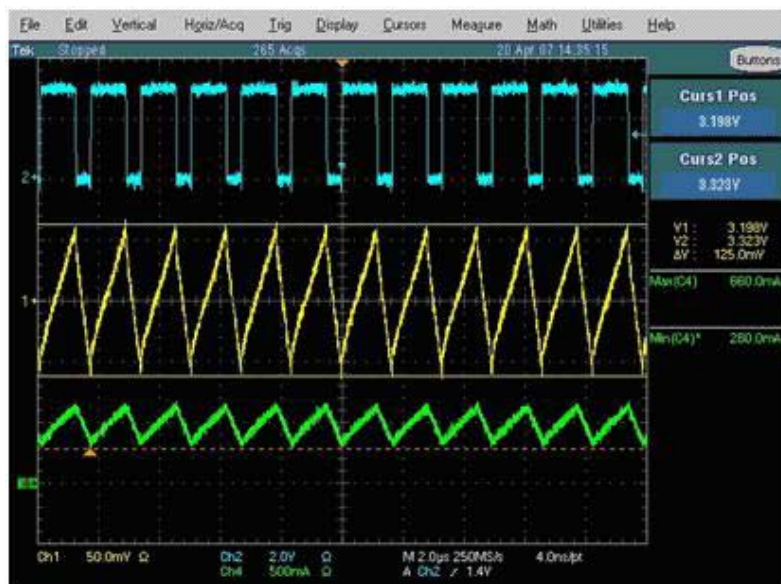
Figure 21. Electrolytic 100 \mu F (Ripple Too High)
