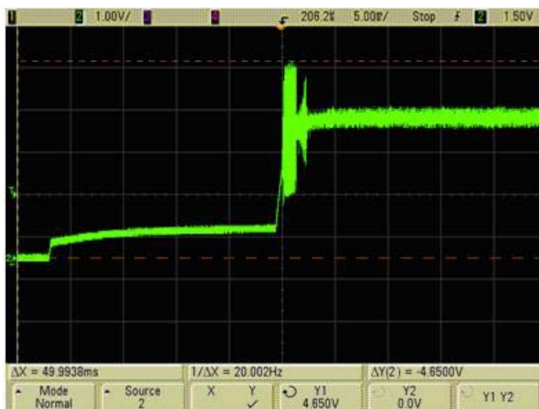
Figure 13. Input Voltage Overshoot >4V (Bad)
